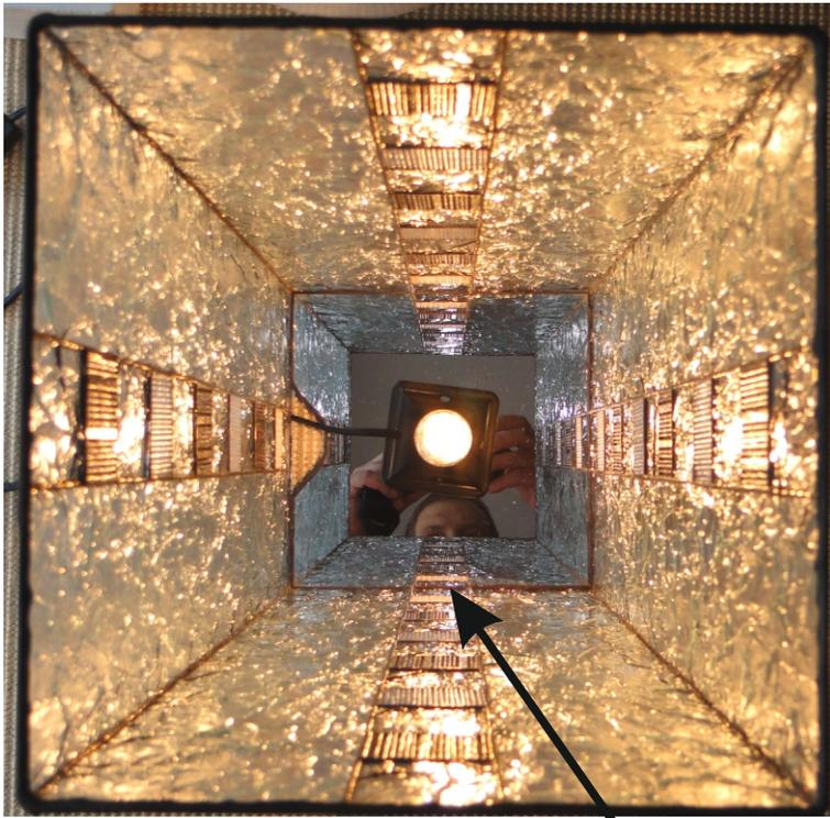
At the upper edge please solder a 2mm brass tube or a sturdy wire for reinforcement.
