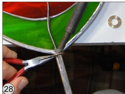
Now slide one of the brass washers up to the joint of the metal structure and solder them together as shown. This transforms the "Breaking point" into a stable and safe construction.
