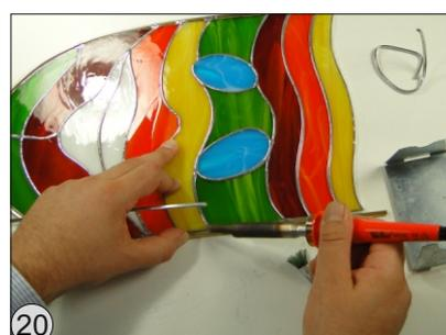
Join the metal frame to the glass work with dots of solder.
