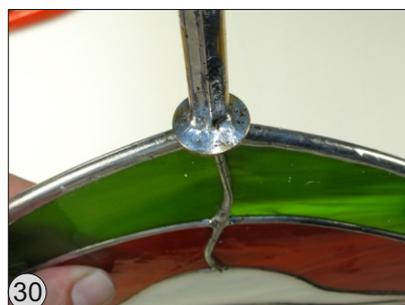
Keep the underside of the washer joint clean so it fits neatly into the pipe later.
