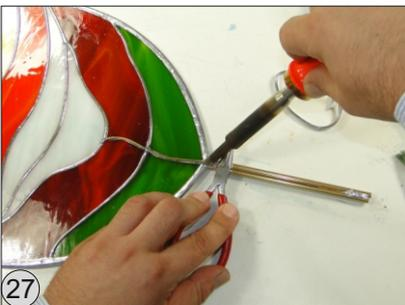
Turn the piece over and add a second 2mm tube to the other side. Both sides of the glass must be stabilized in this way!
