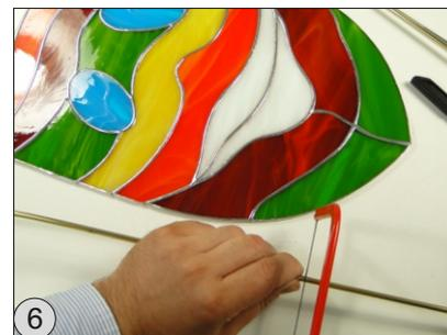
Cut two 15cm lengths of the 5mm brass pipe.
