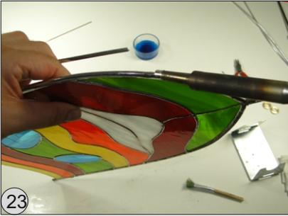
Holding the soldering iron in a horizontal position keeps the liquid from pouring out too quickly.
