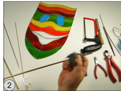
Use steel wool to remove oxide and any rough spots on the pipe to make soldering easier.
