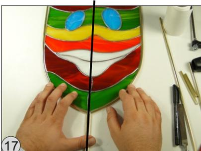
In order for the glass image to stand STRAIGHT in the holder, you should adjust the metal frame properly, before you start soldering it! Later corrections are more difficult ..
