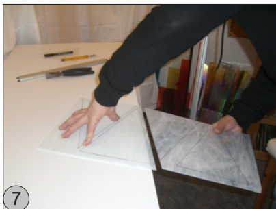
.this is the .. cut point just above the Edge of the table - press the free end of the glass strip down slightly .. cracking - the average is open ...
