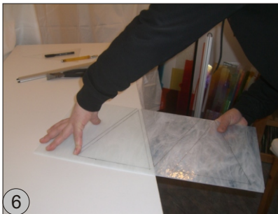
After you scribed the Interface with the glass cutter, just break the Glass strips on the work surface
