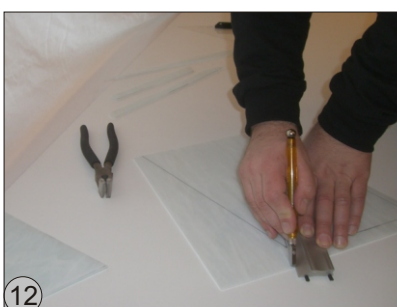
when cutting along an angle or ruler, set the glass cutter above the cutting area and pull the towards you.
