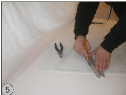
Cut the Glass along a stable ruler. ! Along the straight edge run the Glass cutter towards you!
