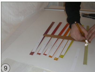
Adapt the glass stripes in the length roughly to the pattern (leave stripes approx. 2 cm longer than pattern).
