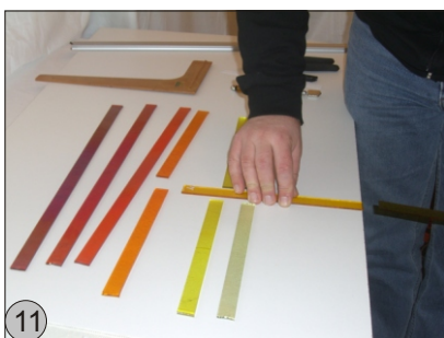
... therefore the cut place lies exactly about the table edge - press the free end of the glass stripe light down. crack - the cut is opened...
