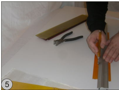
Cut the glass along a stable ruler. !! Along the ruler you lead the glass cutter towards your body !!
