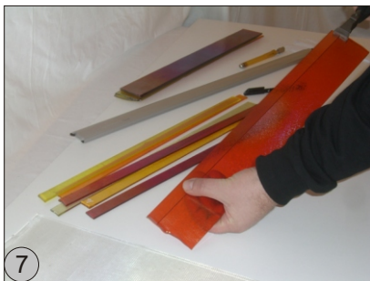
Light pressure of the pliers is enough to open the cut.
