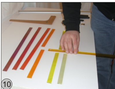
After you have cut the cutting line with the glass cutter, break the glass stripe simply at the working surface.
