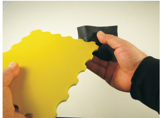
Deburr the edges with wet sandpaper. With wet sandpaper you can regrind also the ground surfaces again.
