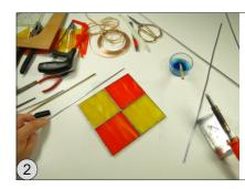
The first step is to remove with thin layer of oxide from the metal strip and brass tube, using steel wool. Simply rub the steel wool all over the metal strip and brass pipe, until everything is blank...
