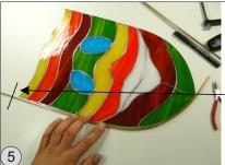
When you have bent the metal to the shape of the glass, the upper end can be marked to saw off.
