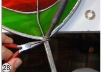
Now slide one of the brass washers up to the joint of the metal structure and solder them together as shown. This transforms the "Breaking point" into a stable and safe construction.
