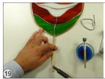
Holding the two straight pipes tightly together, join them at the bottom with a solder dot.
