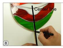
Center Line - Lay the straight metal tube left-justified onto an imaginary center line.
