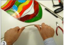
A 5mm brass tube is very stable, but can easily be bent, without the aid of any tools.
