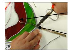
Mount the 2mm tube \_at the first end of the soldered seam.
