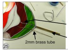
Bend the 2mm brass tube to follow the shape of the center solder line (in the glass panel) then down the length of the straight 5mm brass tubes.
