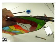
Holding the soldering iron in a horizontal position keeps the liquid from pouring out too quickly.
