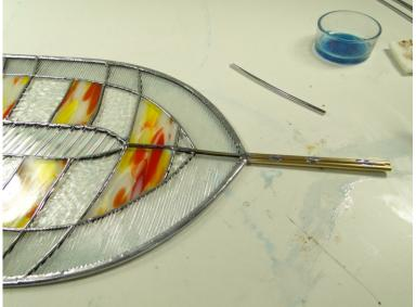
The principle is simple .. Reinforce the glass work with a strong metal frame then add a pipe for a stand and you're all set.
