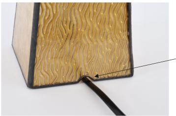
Grind or crumble a small channel on one side for the cable passage.
