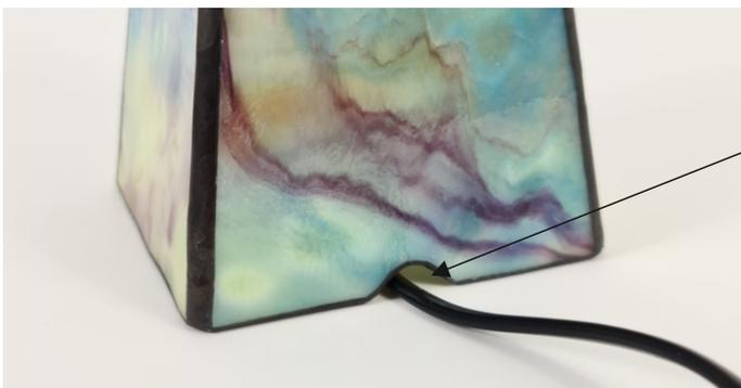
Grind or crumble a small channel on one side for the cable passage.
