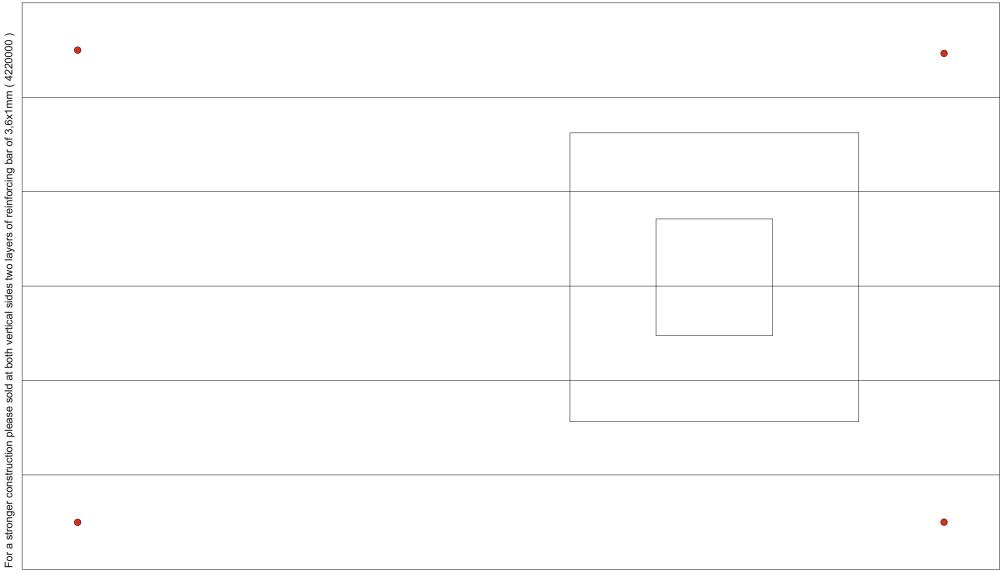
= here you drill a hole of about 6-7mm in diameter. You will need the four holes, for mounting the glass picture onto the wall.
