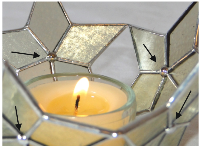
Decorate the center of the stars outside and inside with a small drop of solder.
